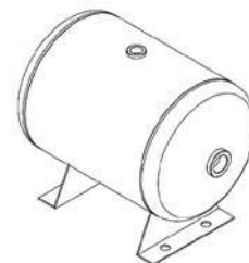
STC TANK brackets welded on the shell
